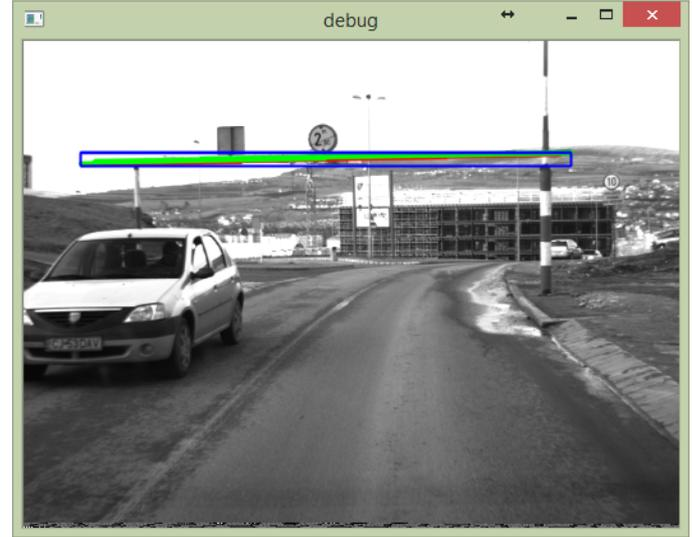
Figure 5. Height restriction barrier bounding rectangle (with blue color); detected barrier lines (red color); valid candidate lines (green color)
