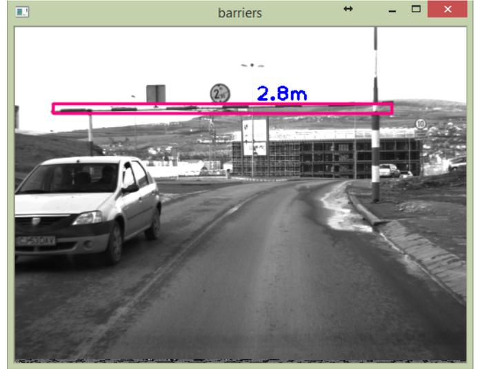
Figure 7. Tracked height restriction barrier (bounding rectangle with magenta color) of the detected barrier from Figure 6
