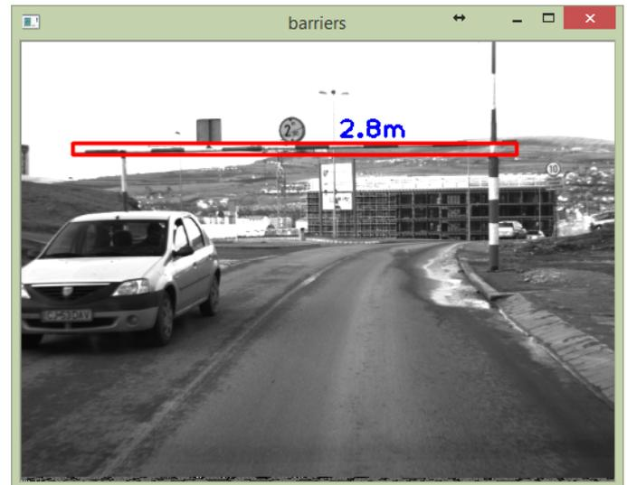
Figure 6. Detected height restriction barrier (bounding rectangle with red color) with the specified height above (with blue color)
