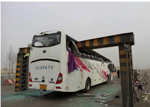
Figure 1. Coach collision with a traffic height restriction barrier in Tianjin, China [1]
